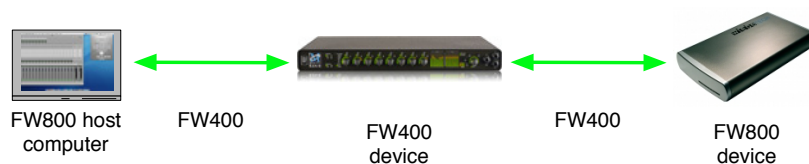
Figure D.2: Incorrectly mixed chain FW800/400
