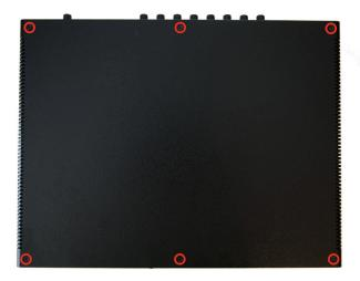
2) Remove the screws from the left and right sides of the case. If the rack ears are fitted, there will be five screws per side. Please note that the screws on the rack ears are longer than the others. Be sure to put the longer screws back in the rack ears when you reassemble the LIO-8.
