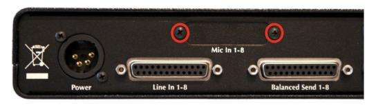
4) Put the DB25 connector board into the LIO-8 so that the connector comes through the hole that you just uncovered. Put the two 7/16" standoffs through the rear panel and screw them into the DB25 connector.
